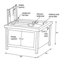
Students discover variables that can be modified affecting the results: Depth of water, weight of pulley, weight of canal boat, shape of canal boat, loading of canal boat. They ultimately discover whether boats travel faster in deeper or shallower canals.
