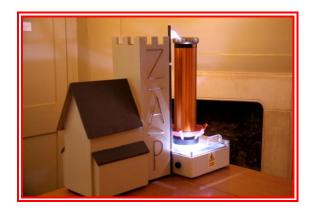
To demonstrate the 18<sup>th</sup> century challenge of protecting buildings from lightning, which Franklin addressed, a model church (with a metal wire running from top to bottom) is used. When placed close to the Tesla coil, sparks strike the church and 'zap' the building. Children then discover Franklin's ingenious solution of the lightning rod, and in so doing, experience a clear, visual demonstration of the difference between electrical **conductors** and **insulators**.
